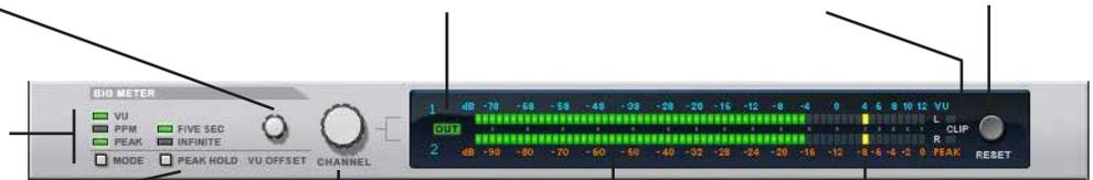
**Channel Select Rotary:** This rotary selects the appropriate Audio Channel from the Hardware Interface, so that it shows up in the metering on the Big Meter Display. Alternately, you can select the appropriate Channel by clicking the Channel Select Button (small square below the corresponding Audio Input / Output Channel pair).
