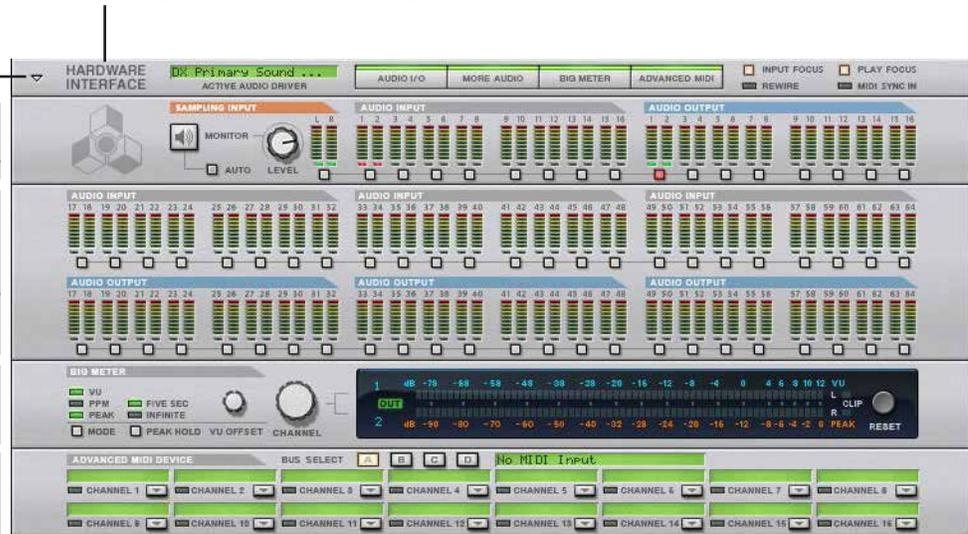
**The Big Meter:** This panel lets you meter any audio In / Out or Sampling Input. This panel is explained in greater detail on the next page.
