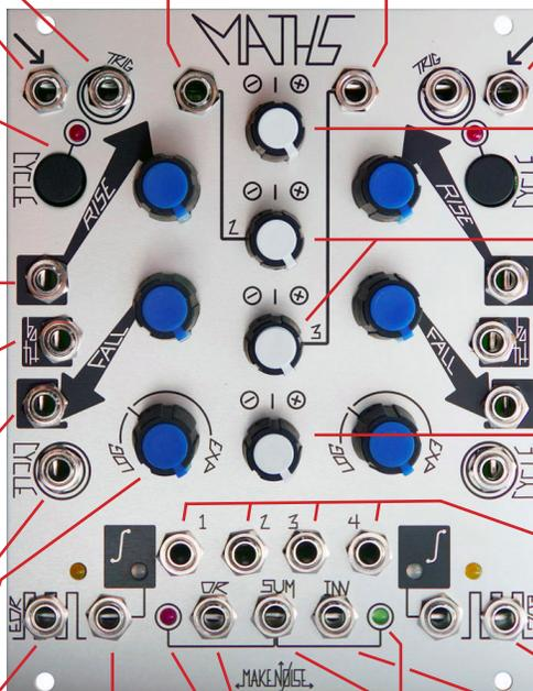
**CHANNEL 1 ATTENUVERTOR ROTARY:** Provides for scaling, attenuation and inversion of the signal being processed or generated by channel 1. Connected to **Channel 1 Variable Out** and **SUM/OR** bus.
