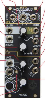
**WOGGLE VCO OUT:** Square Wave audio rate signal, controlled by Woggle rotary control, External In, Ego/Id Balance rotary, Influence CV In, and Clock Speed rotary. 10Vpp.
