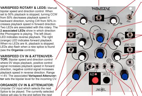
RECORD BUTTON & LED: Manual, momentary button to toggle record on/ off. The Record LED indicates when recording is taking place. When not lit, recording is not taking place.
