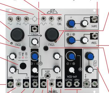
us VCO B 1V/ OCTAVE CV IN: Bipolar pitch control for VCO B. Optimal range: +/-5V.
